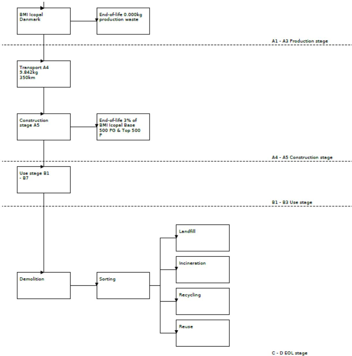
LCA process diagram according to EN 15804 (7.2.1)
