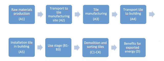
LCA process diagram according to EN 15804 (7.2.1)
