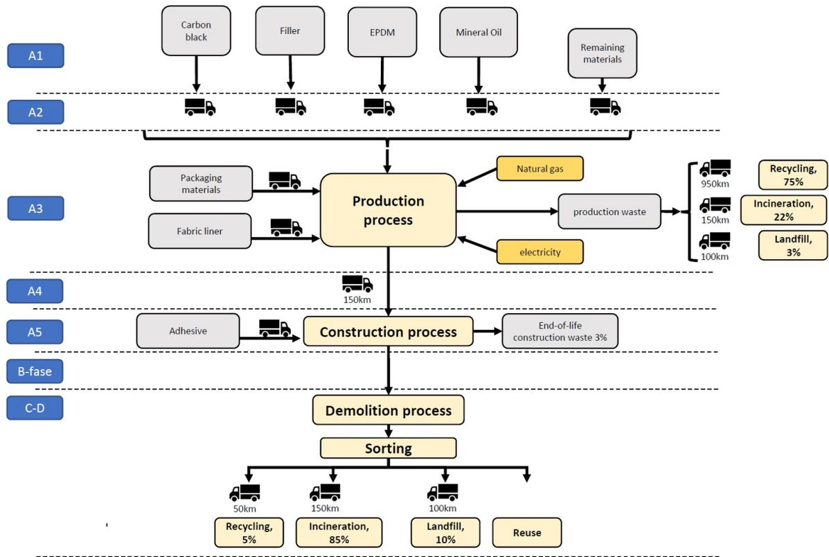
LCA process diagram according to EN 15804 (7.2.1)
