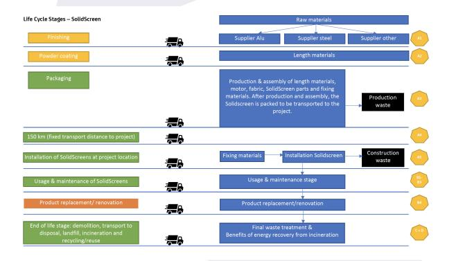
LCA process diagram according to EN 15804 (7.2.1)
