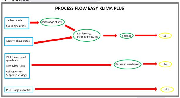
Figure: LCA process diagram according to EN 15804 (7.2.1)
