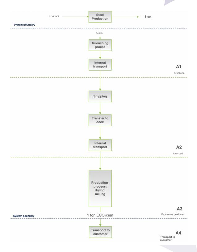
Figure: LCA process diagram according to EN 15804 (7.2.1)
