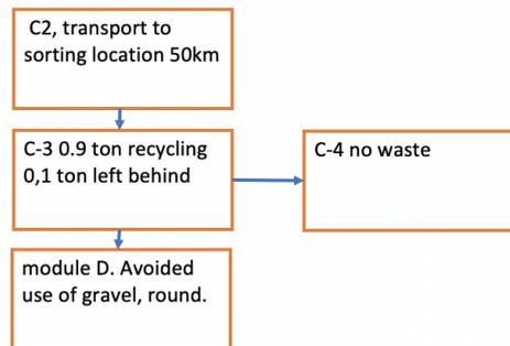
Figure: LCA process diagram according to EN 15804 (7.2.1)
